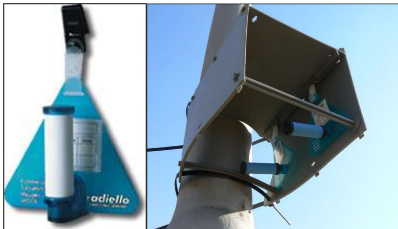
Figure 43: Passive badge sampling equipment
